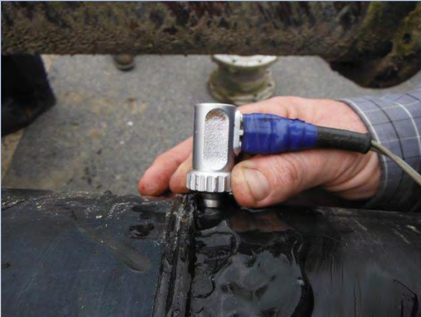
In-Line Transducer for Low Density Materials
