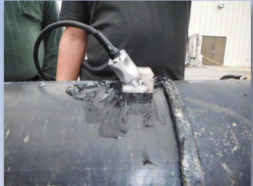
Phased Array Transducer for Testing against Obstructions
